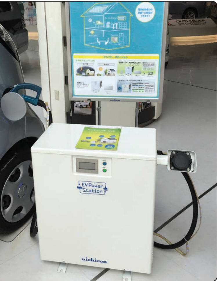
The Nichicon Power Station provides energy from a Mitsubishi Motors i-MiEV directly to a home's electrical system. Nichicon also makes a similar unit for the Nissan Leaf EV.
