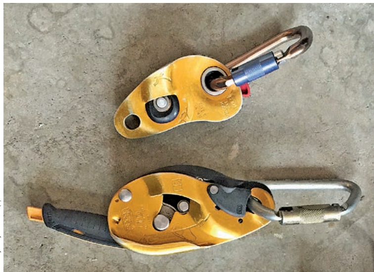
The Petzl I'D can be used for a multitude of things, such as Z-haul and fall-restraint systems, but its main purpose is controlled descent. The I'D Traxion pulley pictured has a one-way stop for hauling heavy items.
